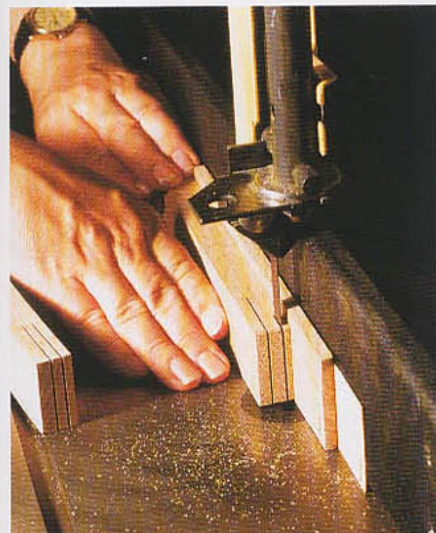
Bridle joints: Use both shims to cut the inside of the tongue
