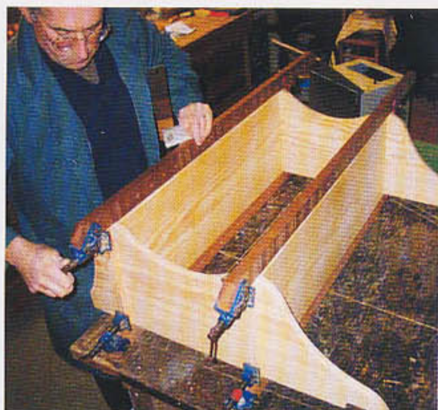
The unit is cramped up and checked for square
