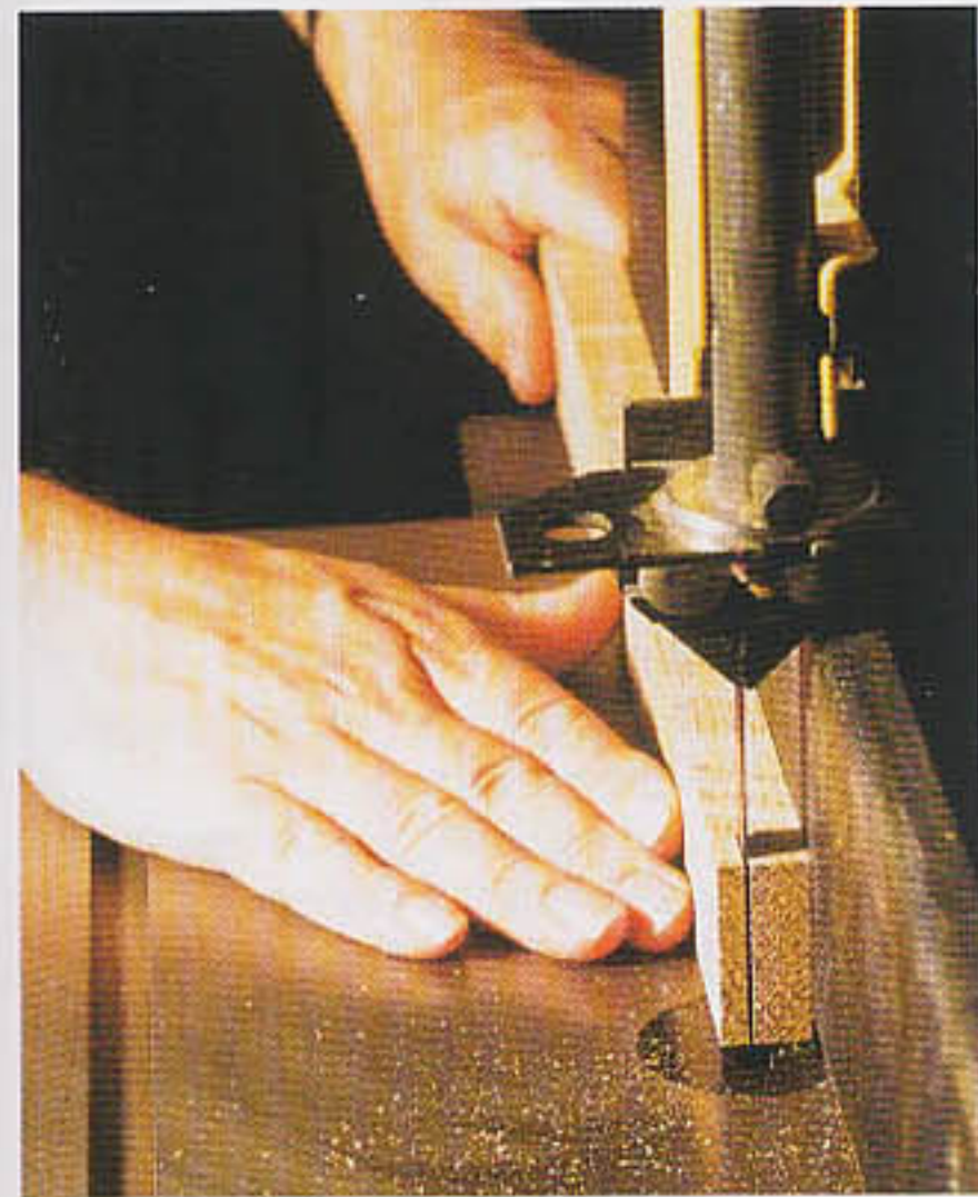
Bridle joints: Run the timber along the fence while cutting the outside of the tongue
