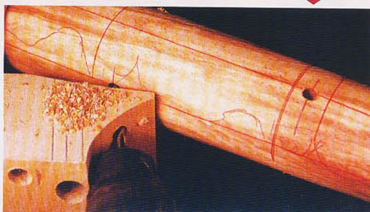
Drill the holes for the mug supports using the drill jig
