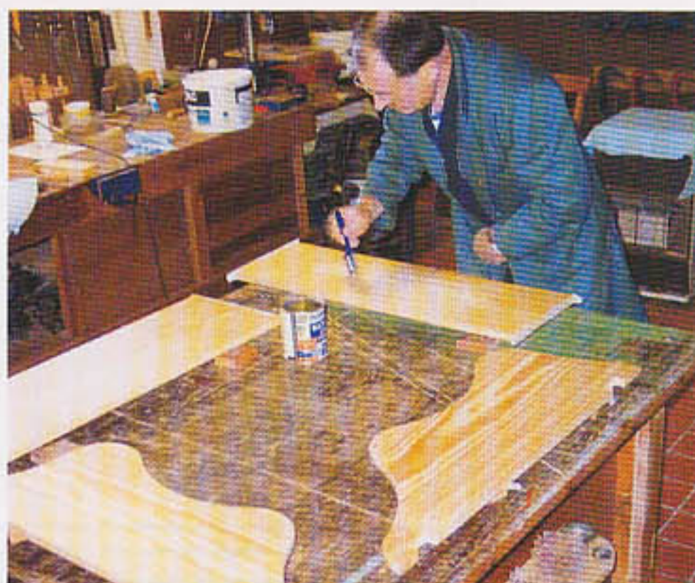
A first sealing coat can be applied before assembly
