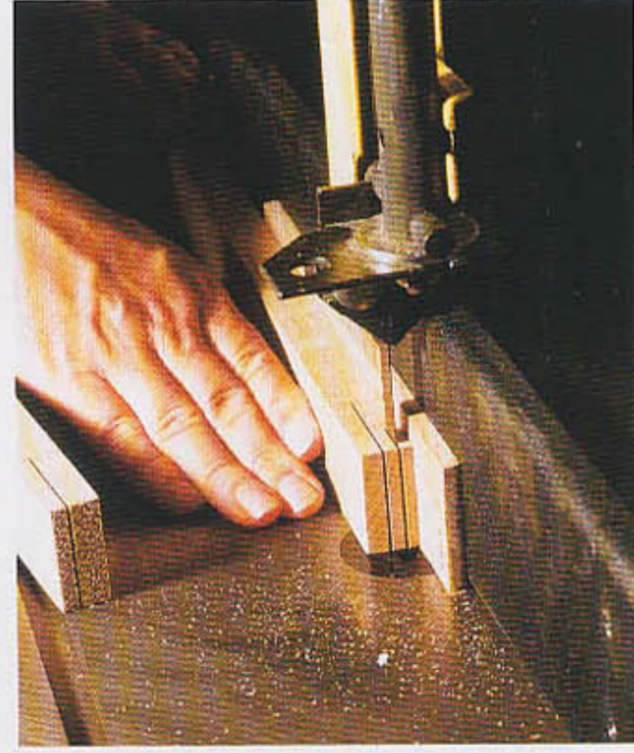
Bridle joints: Cut the inside of the slot with a shim of chisel width
