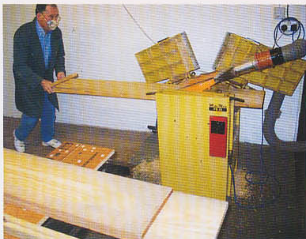
Planing to thickness the wide boards. Look carefully at the stack in the foreground and see how much "cup" had to be planed out!
