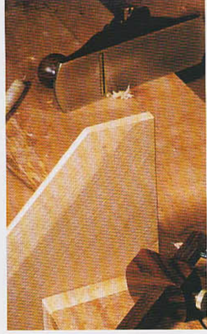
Preparation: Shelves are chamfered with a smoothing plane
