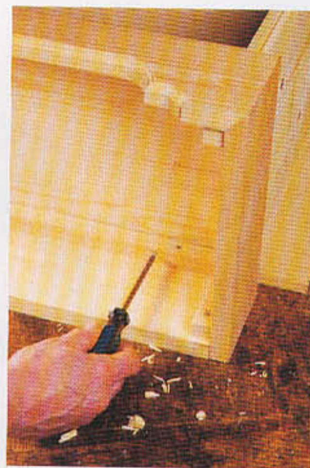
It's a good idea to use a spacer to support the back whilst screwing on the plinth
