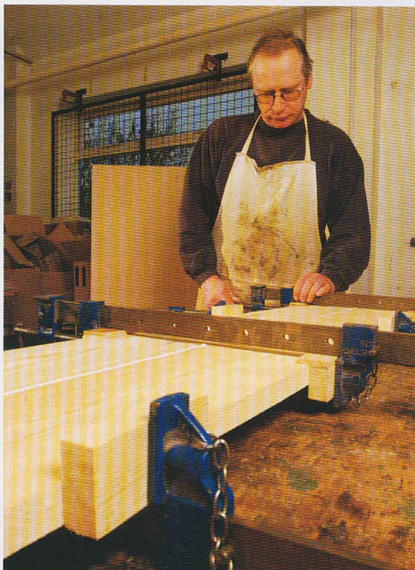
Each side is clamped using sash clamps set up alternating top and bottom to keep the boards flat
