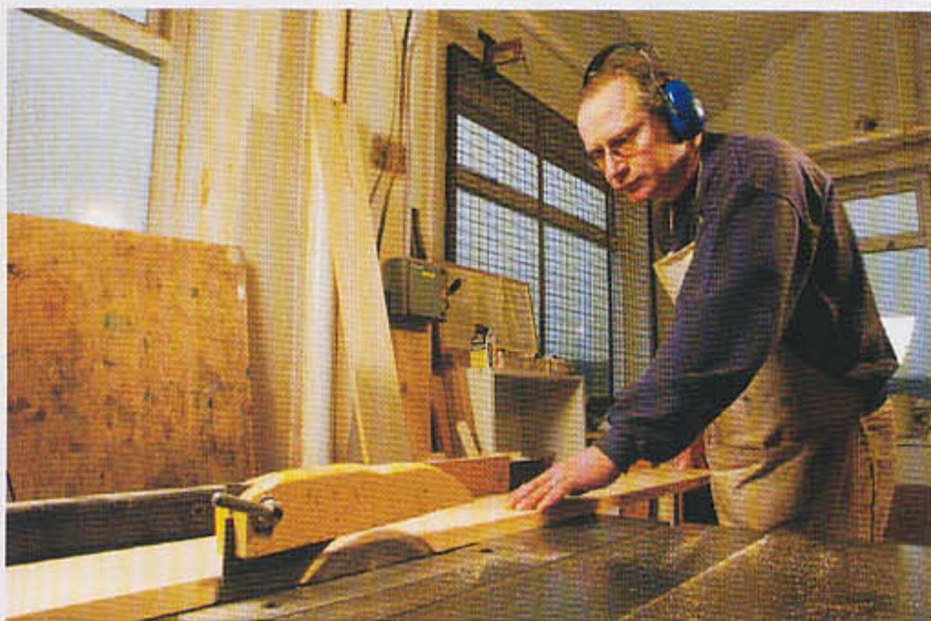
The sides will need sawing accurately before planing the edge joints
