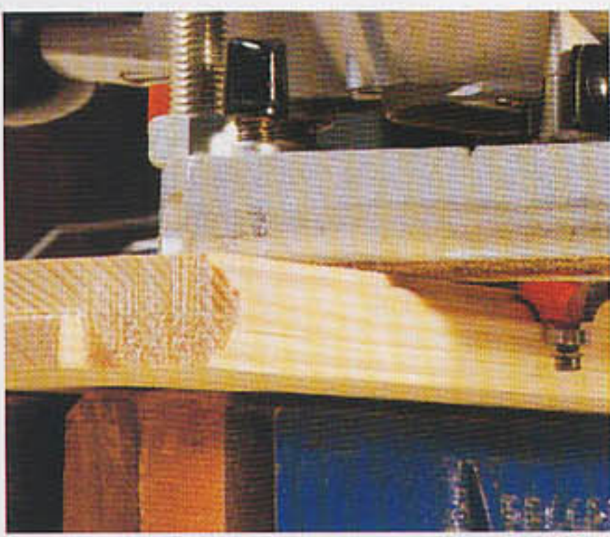
Each shelf has a decorative ovolo mould applied to the top and bottom edges...
