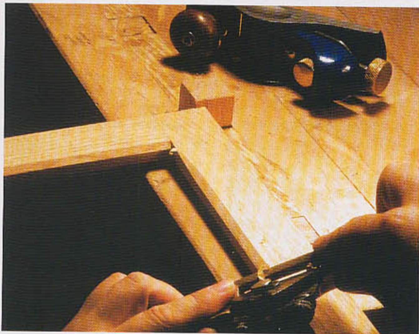
Finishing: Shaving inside chamfers
