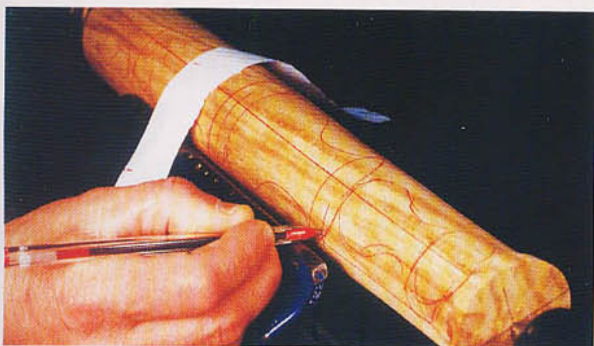
Mark out the peg holes
