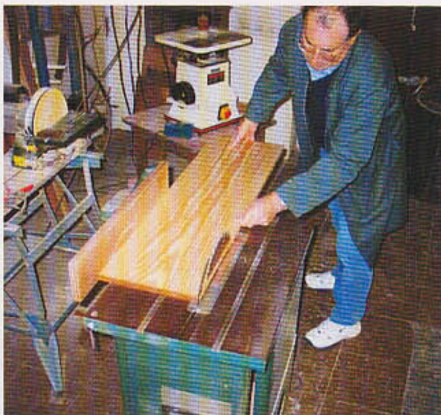
Too wide to be planed to width they are cut accurately on the rip saw bench
