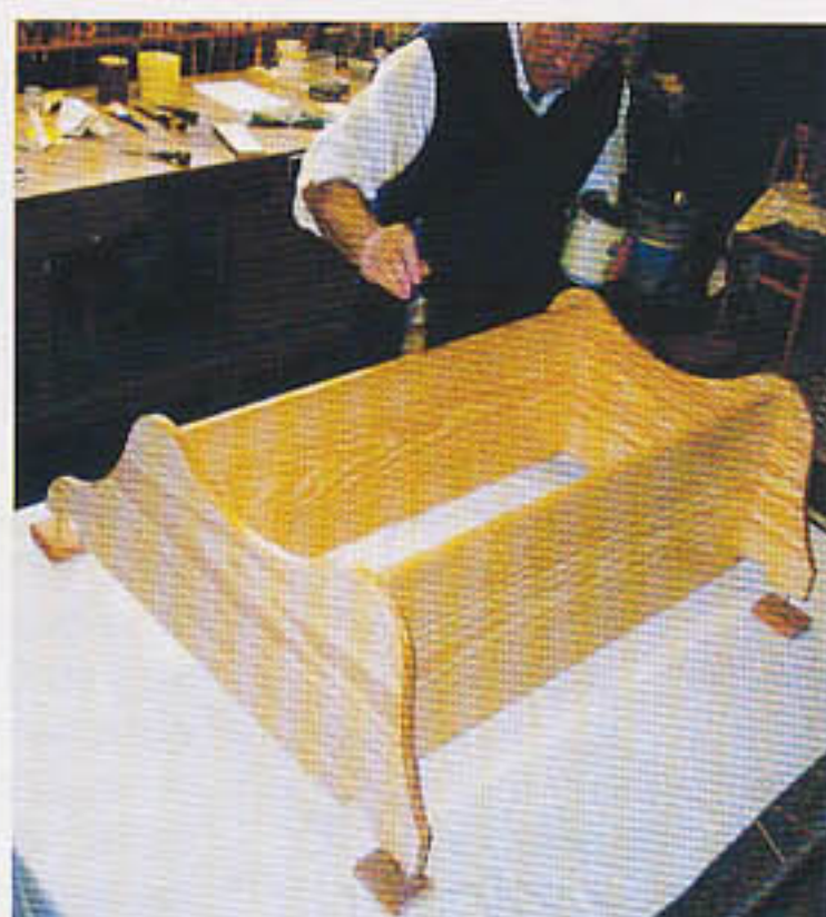
The assembled unit has a second sealing coat
