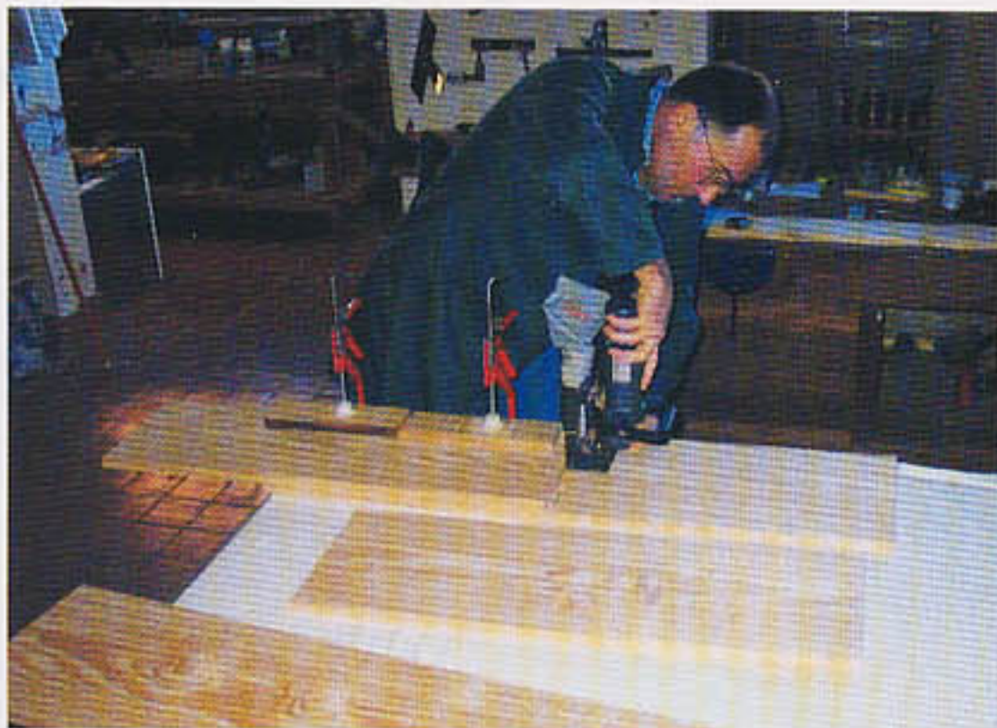
Cutting the joints before shaping takes place
